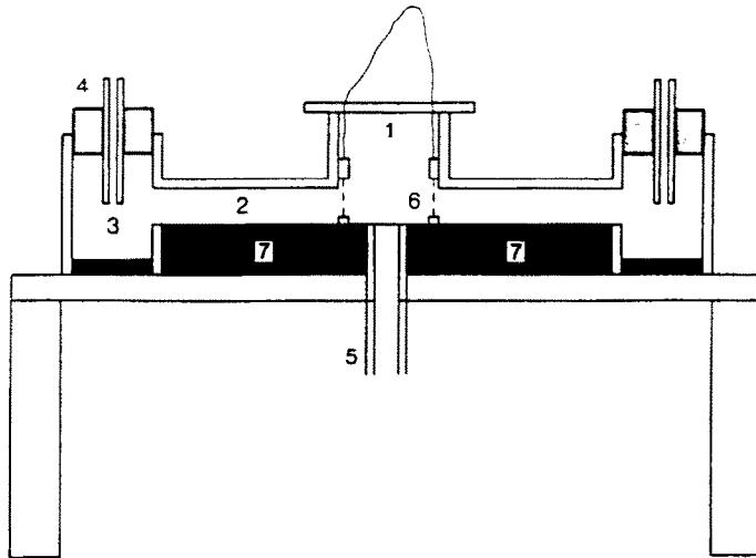
Fig. 1. Olfactometer design. 1. Central chamber. 2. Side arm. 3. Side-chamber. 4. Air inlet. 5. Air outlet to suction pump. 6. Inner ring with plastic net. 7. Plaster of Paris layer.
