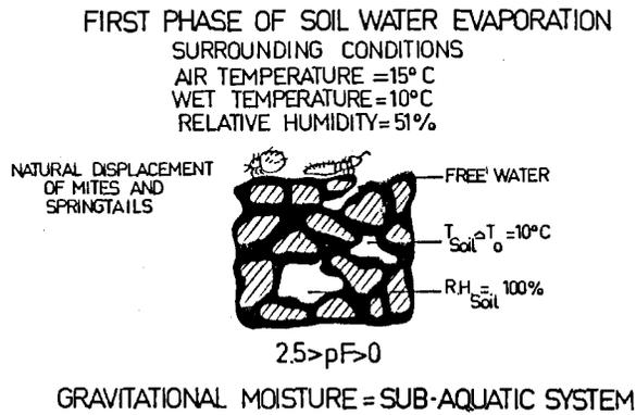
Fig. 3. Diagram of gravitational moisture in the soil framework
