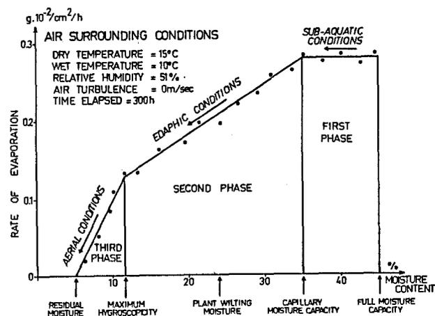
Fig. 2. Curve of unidirectional drying of a moist calcareous soil sample (size,  $20 \times 10 \times 2.5$  cm; wet weight, 700 g). The three phases of the evaporation process illustrate the notion of porosphere: the progressive passage from an aquatic system to an aerial system
