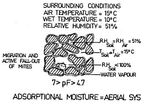
Fig. 5. Diagram of adsorptional moisture in the soil framework
