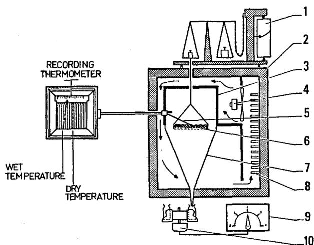
Fig. 1. Schematic diagram of an extraction apparatus for soil microarthropods. 1, recording balance; 2, climate chamber; 3, wind shield; 4, electric fan; 5, thermal probe; 6, sieve with a rectangular slab of soil ( $20 \times 10 \times 2.5$  cm); 7, funnel with steep slides; 8, cooling system; 9, timer; 10, automatic fraction collector recovering microarthropod fallout at 2-h intervals
