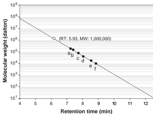
Fig. 3. Estimation of the molecular weight of endo-polysaccharide by gel permeation HPLC with a GFC column. R<sup>2</sup>=0.998. The standard compounds were dextrans with molecular weights of 1.88×10<sup>5</sup> (a), 1.5×10<sup>5</sup> (b), 7.5×10<sup>4</sup> (c), 4.0×10<sup>4</sup> (d), 1.75×10<sup>4</sup> (e), and 1.0×10<sup>4</sup> (f).
