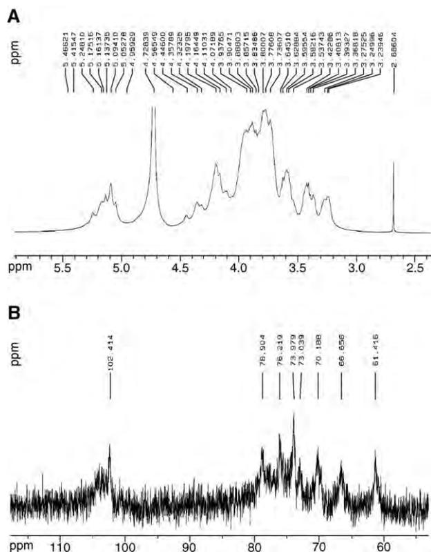
Fig. 5.  $^1\text{H}$  NMR (A) and  $^{13}\text{C}$  NMR (B) spectra of the FII-1 endo-polysaccharide fraction obtained from gel permeation chromatography.
