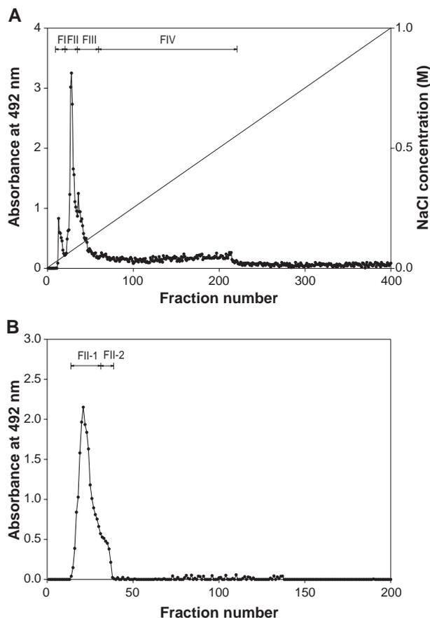
Fig. 2. Elution profiles for ion-exchange chromatography of water-soluble endo-polysaccharide (A), and gel permeation chromatography of FII (B). The straight line in (A) indicates the NaCl gradient. ●: Total sugar content.
