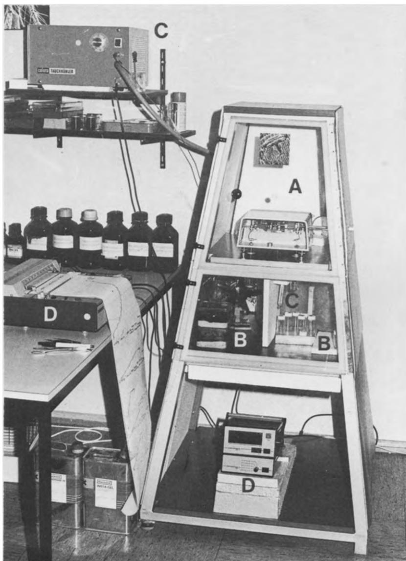
Fig. 1. The ultramicrobalance (Sartorius model 4431), placed in a steel pyramid and connected to a cooling and recording system. Isolation is achieved by aluminium coated styropore plates which can be removed in the front door of the temperature controlled and ventilated area. (A) Balance chamber; (B) Temperature controlled and ventilated area; (C) Cooling system; (D) Recording system.
