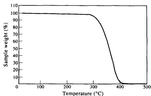
**Figure 5** Thermal degradation of polymer A in air. The heating rate was  $10^{\circ}\text{C min}^{-1}$ .
