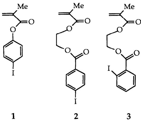
Monomers **1** and **2** could readily be copolymerized with methyl methacrylate (MMA) and/or 2-hydroxyethyl methacrylate (HEMA).
