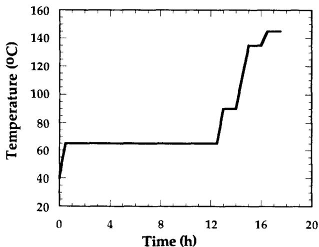
**Figure 1** Time-temperature profile as used in the synthesis of polymers A-C. Cooling at the end of the synthesis was unforced; it took approximately 4 h before room temperature was reached.
