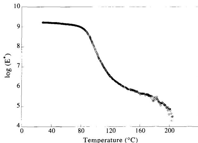
**Figure 6** Results of the DMTA experiments on polymer B. The graph shows  $\log E^*$  ( $E^*$  = dynamic modulus) as function of temperature.
